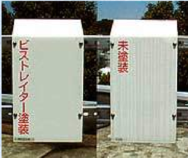
Left: photocatalytic painting Right: normal painting
